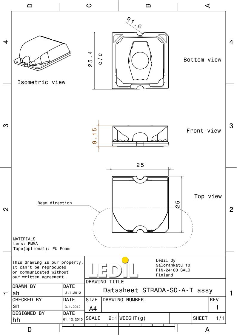
Luminaire: Ledil oy C12410\_STRADA-SQ-A-T-XM-L LOR=88% Lamps: 1 x Cree XM-L 250mA 95lm
