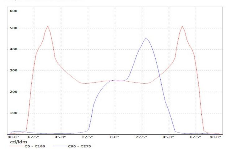
Luminaire: Ledil Oy C12410\_STRADA-SQ-A-T-XM-L Efficiency=93% Lamps: 1 x Cree XM-L 95Im @ 250mA
