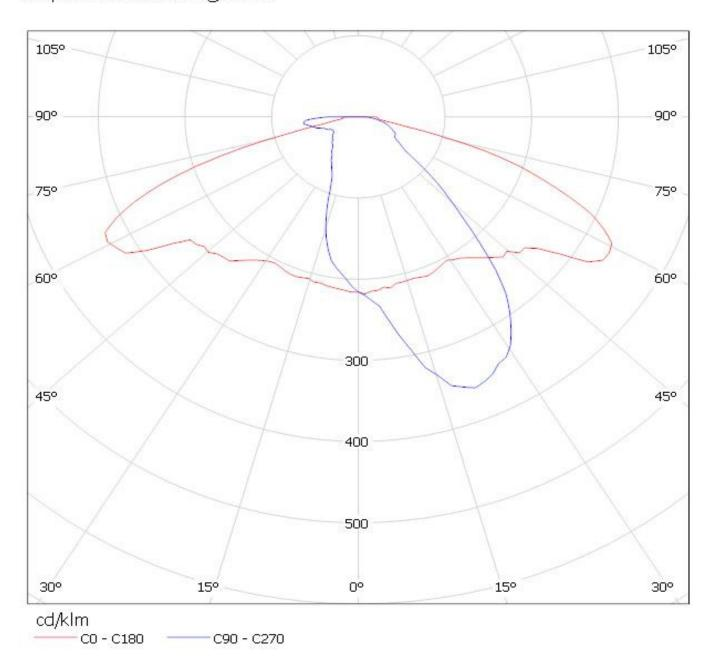
Luminaire: Ledil oy C12411\_STRADA-SQ-A-T-XM-L LOR=88% Lamps: 1 x Cree XM-L 250mA 95lm
