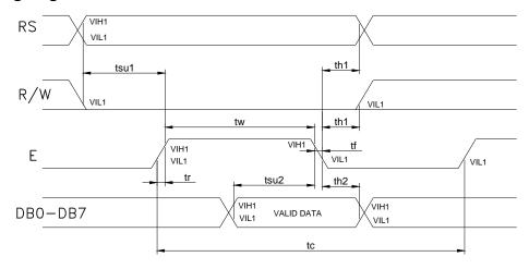
Read cycle (Ta=25 $^{\circ}$ C, VDD=5.0V)
