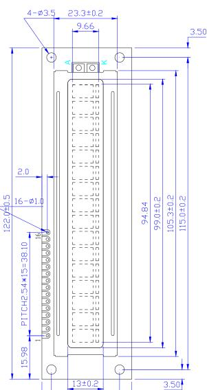
25±0.2 33.0±0.5 Specification: 1). Driving: Duty:1/16, Bias:1/5, VLCD:4.5V, VDD:5.0V 2). Viewing Direction: 6 O'clock 3). Display mode:TN/Positive/Reflective 4). Operating temp.:  $-20^{\circ}c\sim +70^{\circ}C$
