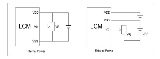
$V_{DD\sim}V_0$ : LCD Driving voltage
