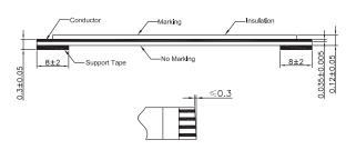
Dimensions: Millimetres Tolerances: ±0.3mm
