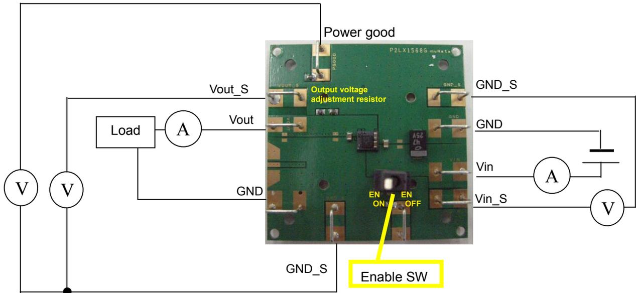
**\* Evaluation board initial output Voltage setting : 3.3V ( resistor : 1.3k $\Omega$  + 12 $\Omega$  )**
