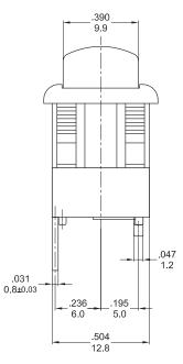
Dimensions : Inches/Millimetres Tolerances ±0.012"/0.3mm
