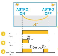
\*Note 3: Depending on the time of year (summer specifically) it may be that the override ON time will fall after the AstroOFF time. In this case, the output switches off at the Astro OFF time and the override ON time is ignored.
