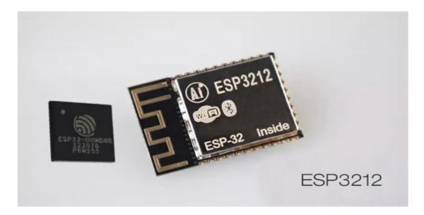
ESP3212 Wifi Bluetooth combo module is ultra high performance and ultra low-power consumption Wi-Fi and Bluetooth combo wireless platform based on ESPRESSIF ESP32 chipset. ESP-3212 integrates dual-core processor, 448 KByte ROM,520 KByte SRAM,16 KByte SRAM in RTC, 802.11 b/g/n/e/I Wi-Fi, Bluetooth v4.2 BR/EDR & BLE, clocks & Times, abundant peripheral Interfaces and sercurity mechanism.
