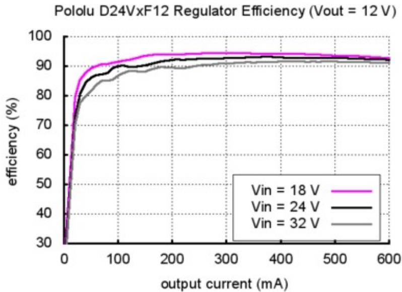
Note that the above graphs apply to both the 300 mA and 600 mA versions, which is why the x axis extends to 600 mA. You should not expect to get more than 300 mA from the 300 mA versions (D24V3Fx). These graphs and ones below do not apply to our newer 500 mA D24V5Fx buck regulators, which have different operating characteristics, including much lower dropout voltages.
