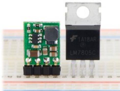
Pololu step-down voltage regulator D24VxFx next to a 7805 voltage regulator in TO-220 package.
