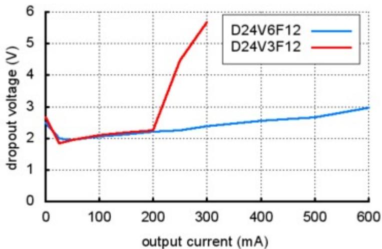
As you can see from the last two graphs, the dropout voltage of the low-current 9 V and 12 V versions (D24V3F9 and D24V3F12) spikes as the output current nears the 300 mA limit. For similar regulators with much lower dropout voltages, please consider our newer 500 mA D24V5Fx
