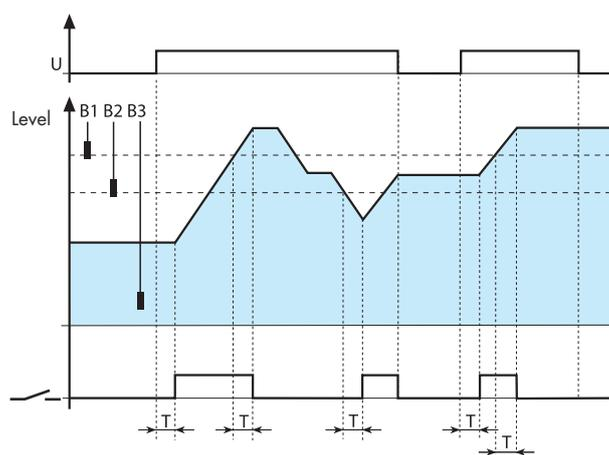
**Filling Control** – between Min. and Max. levels.
