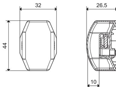
Floor surface water sensor for connection to electrode terminals (B1 and B2) of 72.01 or 72.11 level control relay, set in Emptying function (ES or E respectively).
