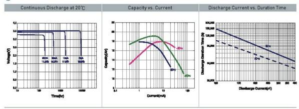
\*\* This data was made on basis of nominal capacity for the purpose of enabling users to forecast approximate life time.
