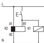
• Possible to control an external load, such as another relay coil or timer, connected to the signal start terminal B1.
