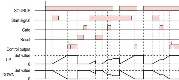
Timing starts when the start signal goes ON.
