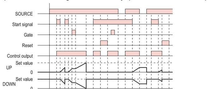
The control output is ON when the start signal is ON(except when the power is OFF or the reset is ON).
