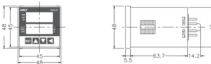
Y type(Flush Mounting): Using Y50 Frame & US-08 Socket , P3G-08 Socket or P3G-11 Socket(for H5CLR-11/11M use only)
