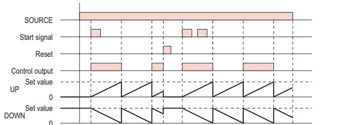
Timing starts when the start signal goes ON.
