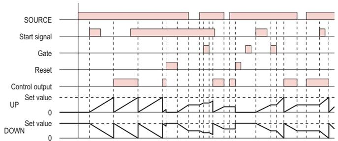
Timing starts when the start signal goes ON.
