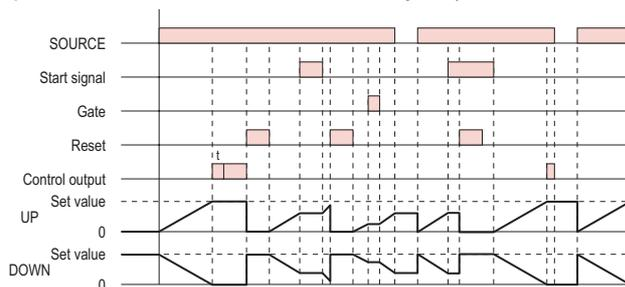
Timing starts when the reset input goes OFF.
