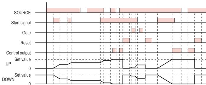
Start signal enables timing (timing is stopped when the start signal is OFF or when the power is OFF)
