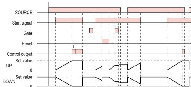
Timing starts when the start signal goes ON, and is reset when the start signal goes OFF.
