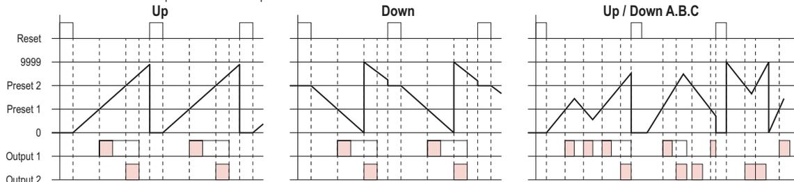
**Output mode P** : Present value display does not change during 1-shot time period, but reset start status is returned to as soon as count is reached. Outputs are 1-shot and operate repeatedly. Output 1 is self-holding, and goes off after expiration of the 1-shot period for Output 2. One-shot time periods for Output 1 and 2 are independent.
