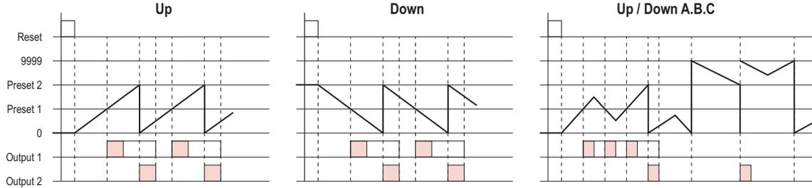
**Output mode R** : Present value is placed in reset start status as soon as count up is reached. Outputs are 1-shot and operate repeatedly. Output 1 is self-holding, and goes off after expiration of the 1-shot period for Output 2. One-shot time periods for Output 1 and 2 are independent.
