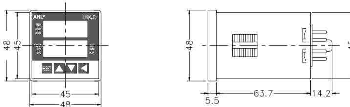
Y type(Flush Mounting): Using Y50 Frame & US-08 Socket , P3G-08 Socket or P3G-11 Socket(for H5KLR-11/11M use only)
