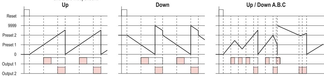
**Output mode A** : Present value and output 1 maintain status until reset. Output 1 and 2 operate independently.
