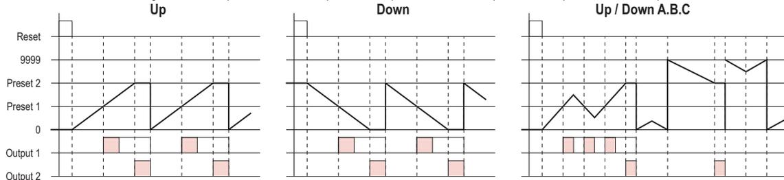
**Output mode K** : Present value runs continuously. Output 1 is self-holding, and goes off after expiration of the 1-shot period for Output 2. One-shot time periods for Output 1 and 2 are independent.
