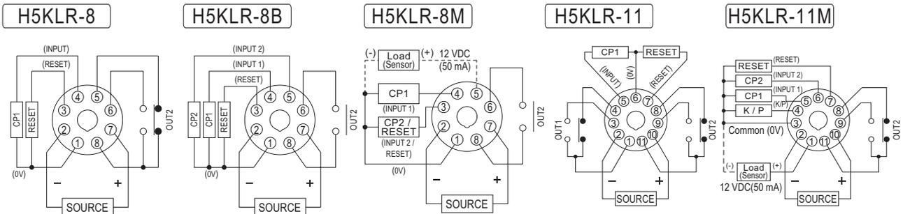
Note: **H5KLR-8** : When using Proximity(Type NPN) or photoelectric switch, connect (+) to external 12VDC, (-) to pin (1) and (OUT) to pin (4). (OUT2) to pin (5) for H5KLR-8B only. Connect (+) to pin (5) and (OUT) to pin (4), (OUT2) to pin (3) for H5KLR-8M only.
