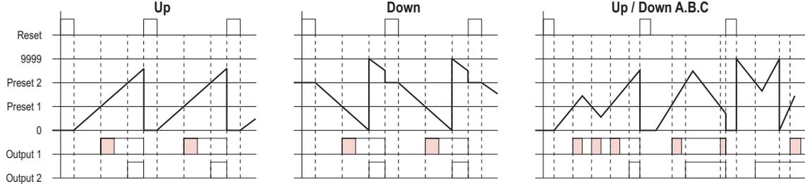
**Output mode C** : Present value is placed in reset start status as soon as count up is reached. The count up is not displayed. Outputs are 1-shot and operate repeatedly. Output 1 is self-holding, and goes off after expiration of the 1-shot period for Output 2. One-shot time periods for Output 1 and 2 are independent.
