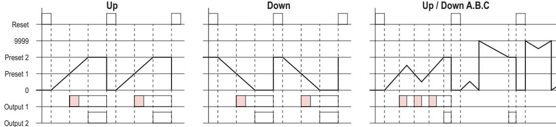
**Output mode F** : Present value display runs continuously. Outputs are maintained until reset.
