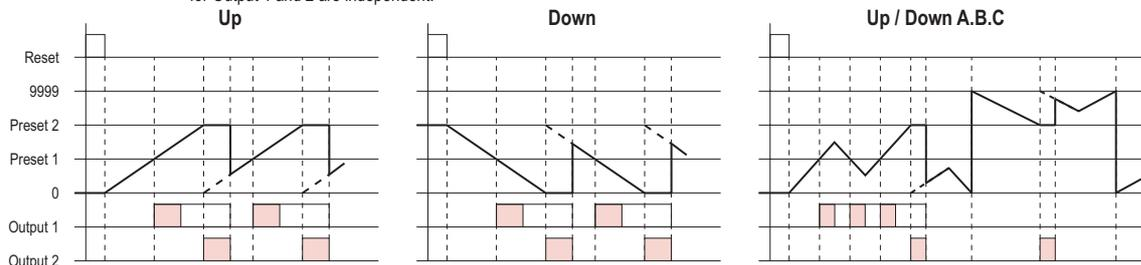
**Output mode Q** : Present value runs continuously through 1-shot time period and returns to reset start status immediately afterward. Outputs are 1-shot and operate repeatedly. Output 1 is self-holding, and goes off after expiration of the 1-shot period for Output 2. One-shot time periods for Output 1 and 2 are independent.
