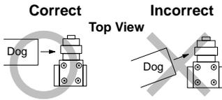
When using a long lever model like the D4B-□□16N or D4B-□□17N, the Switch may telegraph. To avoid telegraphing, take the following precautions.
