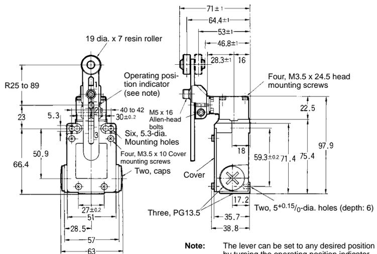
**Note:** The lever can be set to any desired position by turning the operating position indicator.
