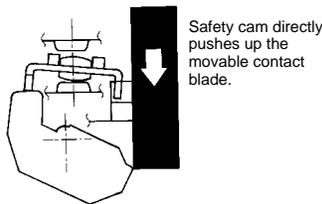
3. When contacts are completely pulled apart.
