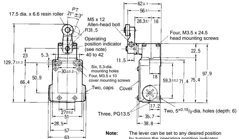
**Note:** The lever can be set to any desired position by turning the operating position indicator.
