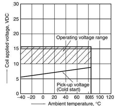
3. Ambient temperature characteristics (Cold/initial)
