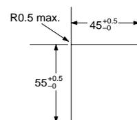
**Note:** The mounting panel thickness should be 1 to 3.2 mm.
