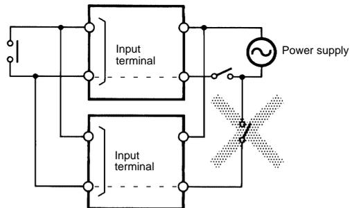
**Relationship between Input and Power Supply Circuits (H3CR-A□/-A□S)**
