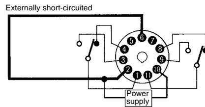
**2. Signal Start/Signal Reset (in B Mode)**
