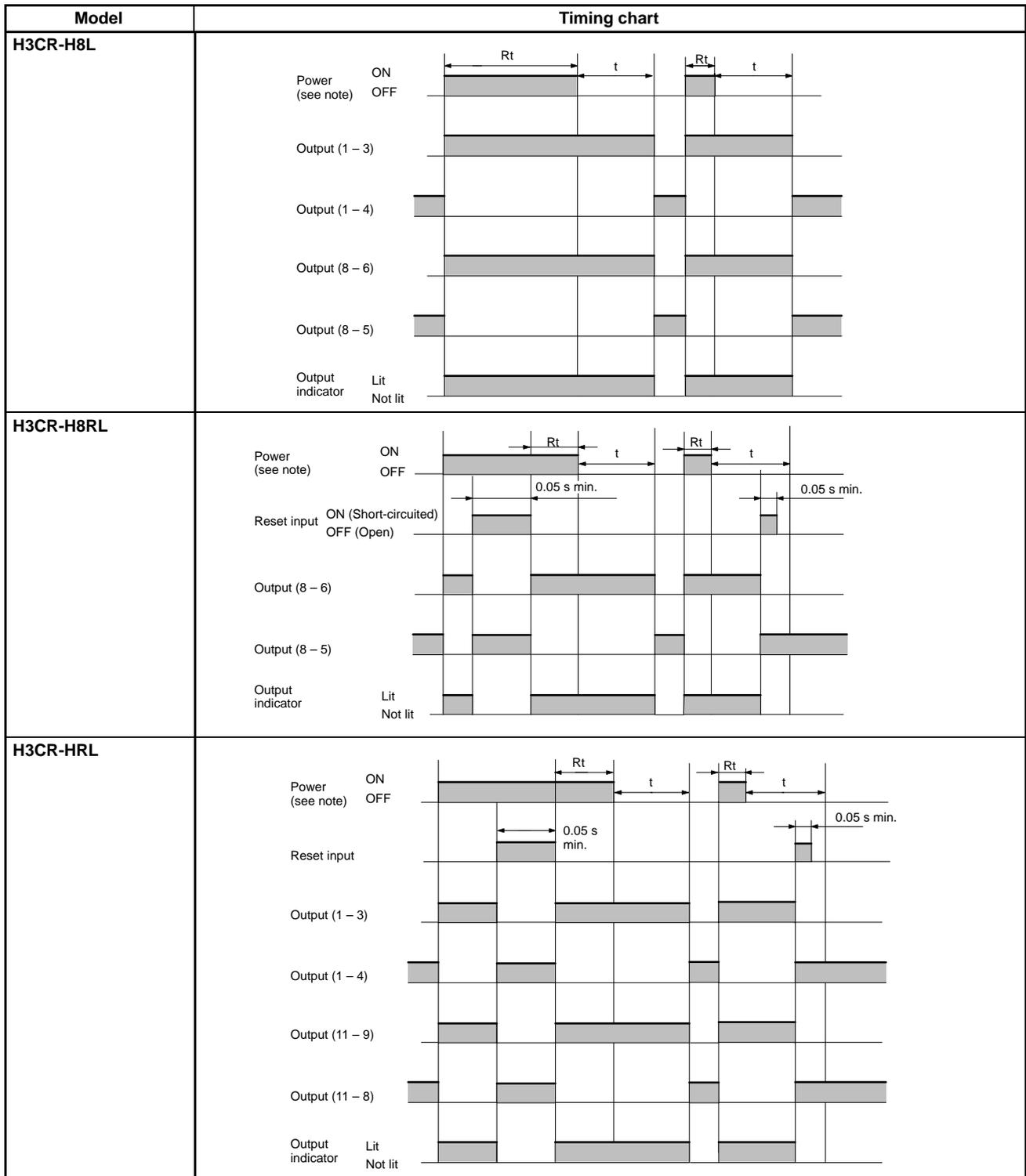
**Note:** If the power is turned ON until the set time is up, the timer will be retriggered.
