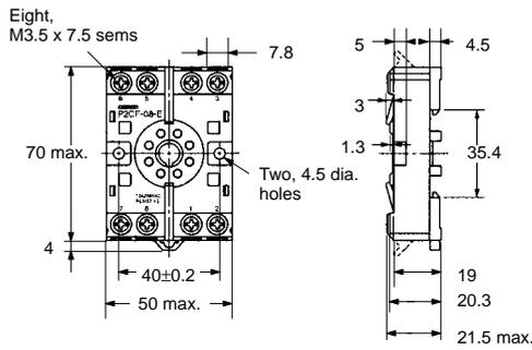
**Track Mounting/Front Connecting Socket**
