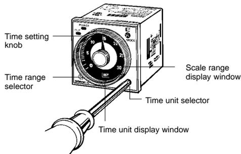
For OFF-time, the desired time unit (sec, 10 s, min, and hrs, or 10 s, 10 min, hrs, and 10 h) is indicated in the OFF-time unit display window at the upper right corner of the front panel and can be changed by turning the OFF-time unit selector located below the OFF-time unit display window.
