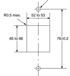
**Note:** The mounting panel thickness should be 1 to 3.2 mm.
