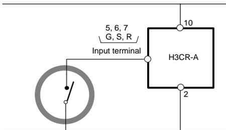
Do not connect a relay or any other load between input terminals, otherwise the internal circuit of the Timer will be damaged due to the high-tension voltage applied to the input terminals.
