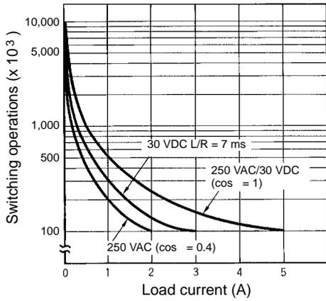
Reference: A maximum current of 0.15 A can be switched at 125 VDC (cos = 1) and a maximum current of 0.1 A can be switched if L/R is 7 ms. In both cases, a life of 100,000 operations can be expected. The minimum applicable load is 10 mA at 5 VDC (failure level: P).
