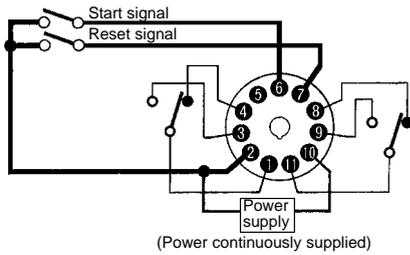
**2. Signal-ON-OFF Start/Instantaneous Operation/Time-limit Reset**
