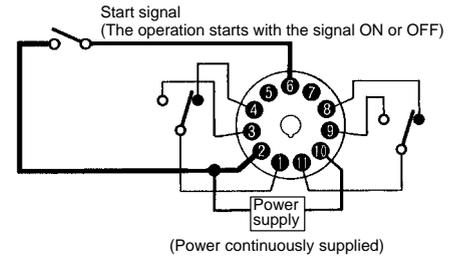
**C Mode: Signal ON/OFF-delay**
