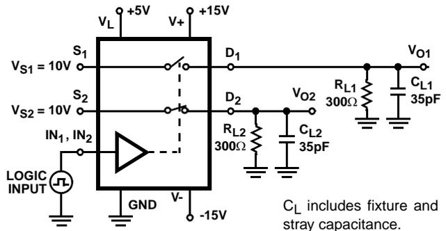
$C_L$  includes fixture and stray capacitance.
