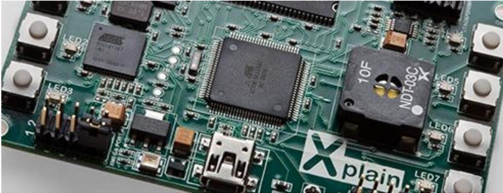
The Atmel AVR Xplained kits are great platforms for early evaluation of the capabilities offered by the Atmel AVR microcontrollers. The XMEGA-A3BU Xplained contain one QTouch button sensor, three mechanical buttons, two LEDs, 3 analog sensors, a USB port, battery backup system and a 128x32 pixel FSTN LCD display.
