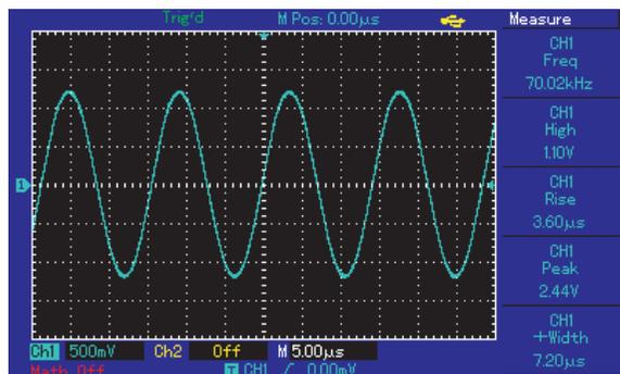
Figure 3-1 Automatic measurement
