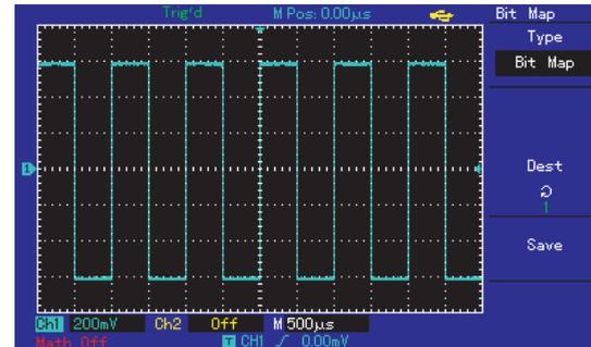
Figure 3-11 Waveform storage
