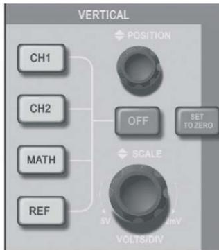
Figure 3-13 Vertical control panel of 5.7-inch screen
