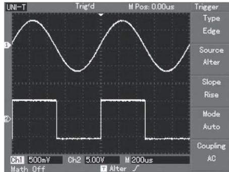
Figure 2—16 Observation of 2 signals with different frequency by.
