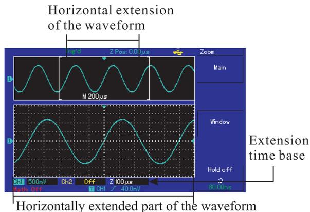
Figure 2—12 Screen display under view window extension
