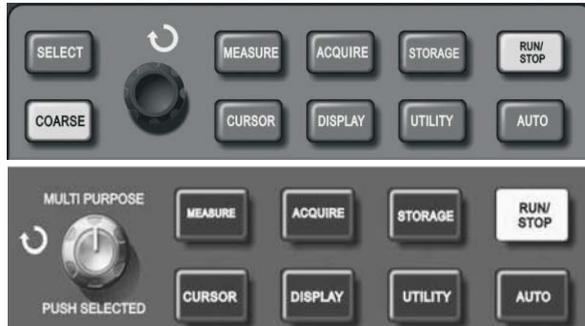
Figure 2-30 Operation/stop key
