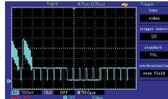
Figure 2-15 Video trigger: Field synchronization ALT TRIG mode
