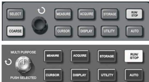
Figure 2—27 Function key (and function) of sampling
