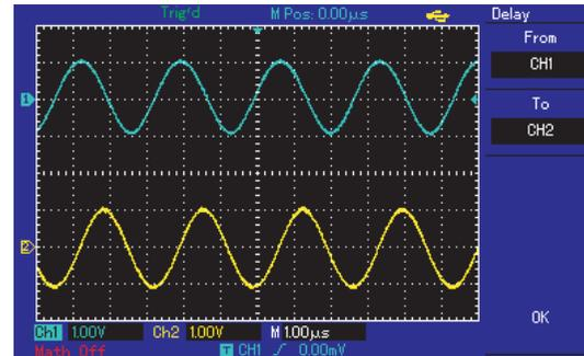
Figure 3-2: Waveform delay
