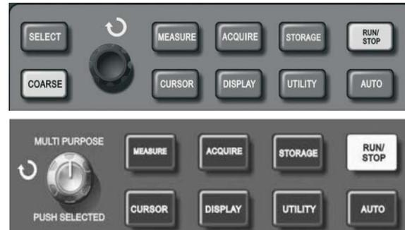
Figure 2-29 Function key (or cursor) of sampling system
