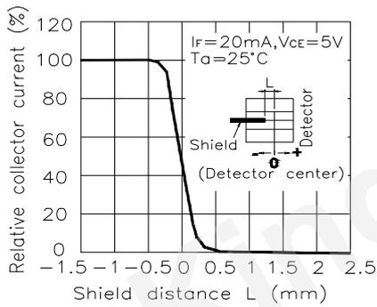
**Fig.7 Relative Collector Current vs. Shield Distance (2)**
