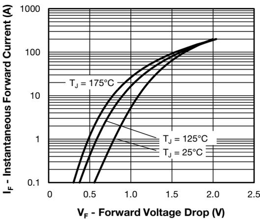
Fig. 1 - Forward Voltage Drop Characteristics, Per Leg
