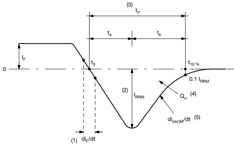
Fig. 13 - Reverse Recovery Waveform and Definitions
