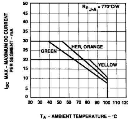
Figure 9. Maximum Allowable DC Current vs. Ambient Temperature.
