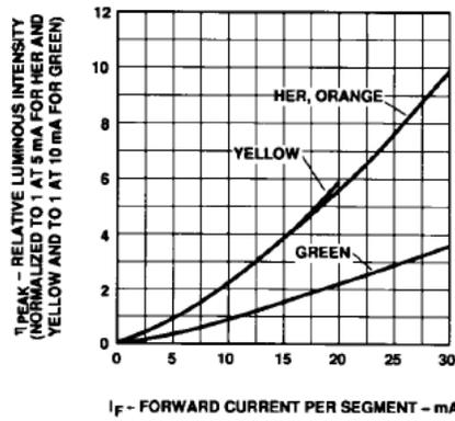
Figure 11. Relative Luminous Intensity vs. DC Forward Current.
