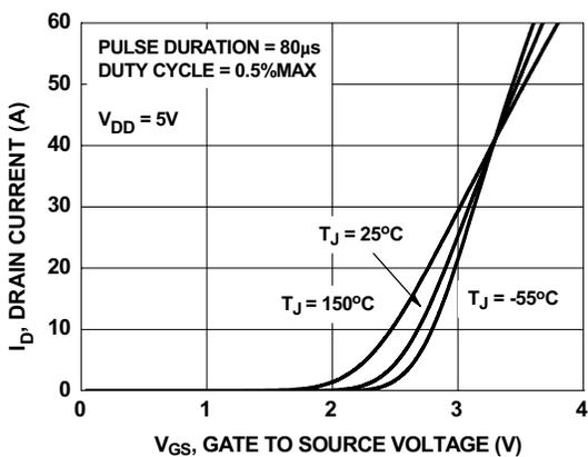
Figure 5. Transfer Characteristics
