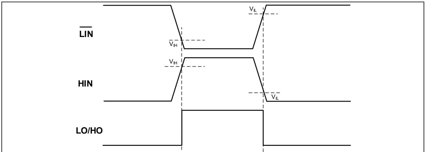
Figure 10 HIN &amp; LIN input thresholds
