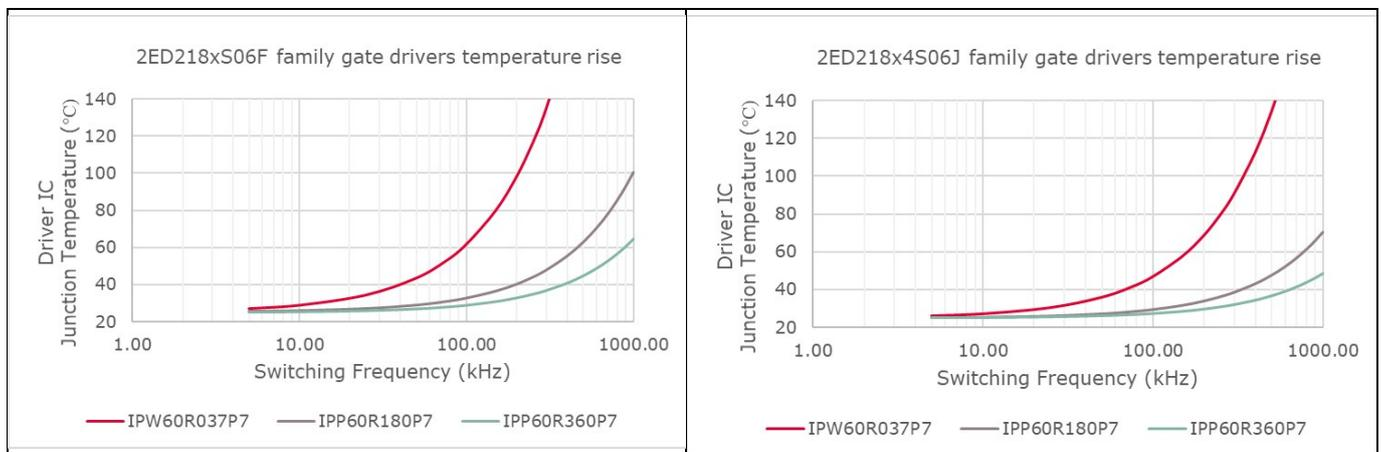
\*Assumptions for above curves:  $T_a = 25^\circ\text{C}$ ,  $V_{BUS} = 400\text{ V}$ ,  $V_{CC} = 12\text{ V}$ ,  $R_{gon} = 10\ \Omega$ ,  $R_{goff} = 5\ \Omega$
