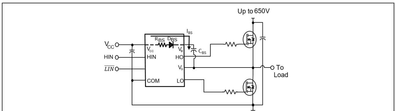
Figure 14 Half bridge bootstrap circuit in 2ED218x
