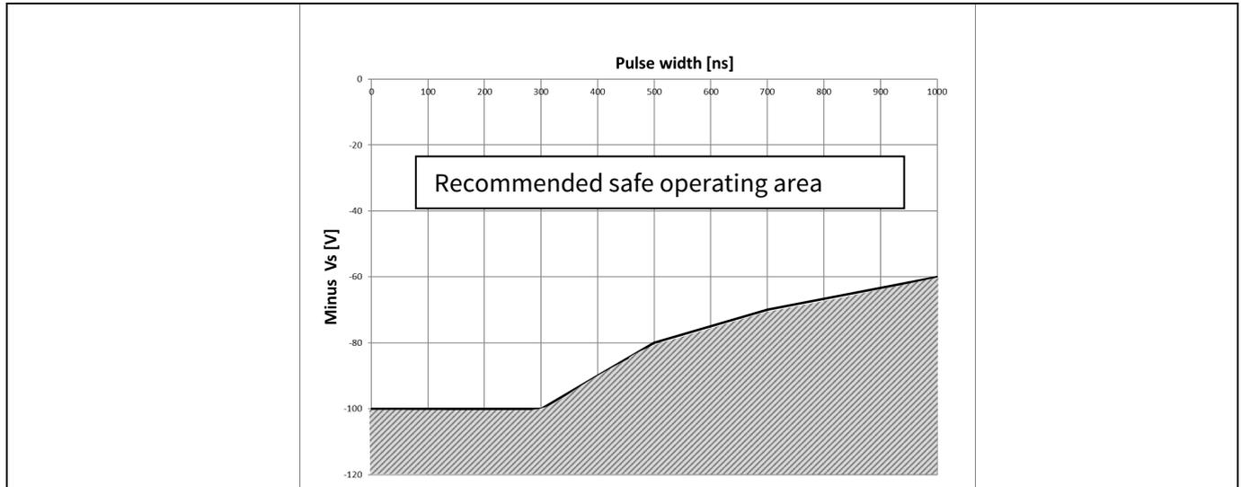
Figure 19 Negative VS transient SOA for 2ED2183(4)S06F(J) @  $V_{BS}=15\text{ V}$
