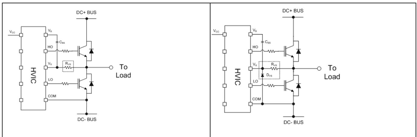
Figure 23 Resistor between the  $V_S$  pin and the switch node
