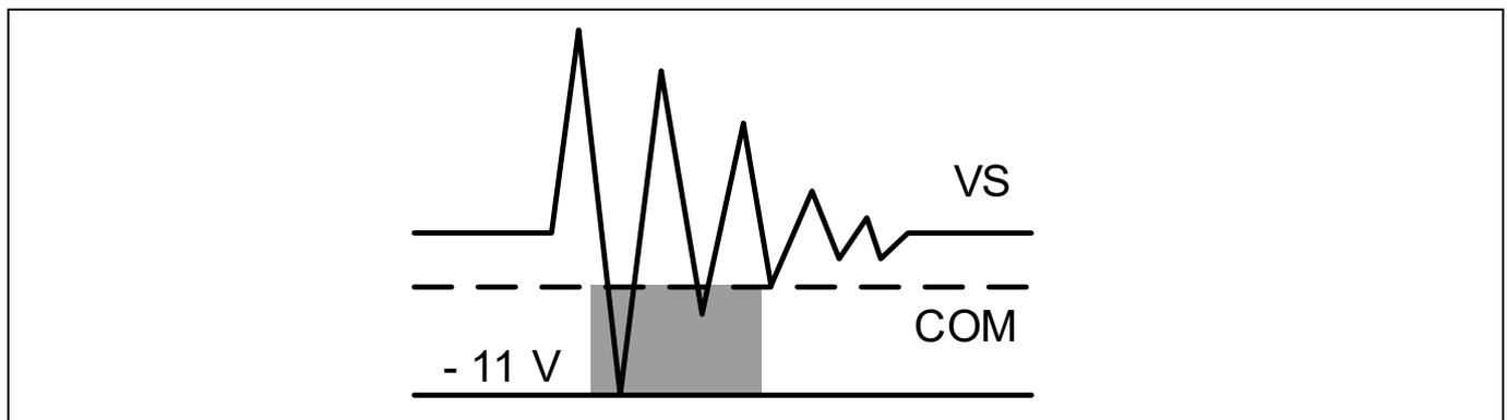
Figure 20 Headroom for HV level shifter data transmission
