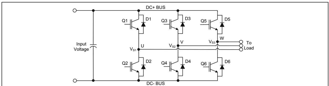
Figure 16 Three phase inverter
