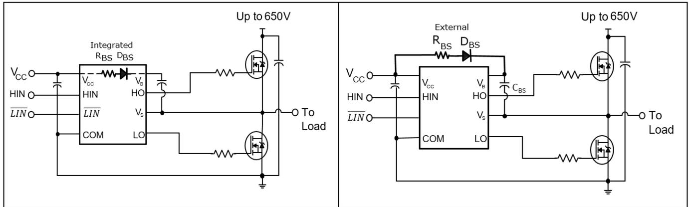
Figure 12 2ED218x with integrated components      Figure 13 Standard bootstrap gate driver
