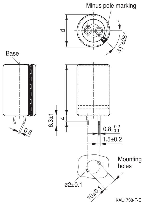
Large-size capacitors, snap-in terminals, length (6.3 ± 1) mm.
