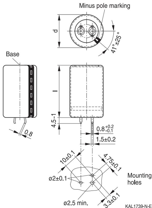
Large-size capacitors, snap-in version with 3 terminals (length (4.5 - 1) mm).
