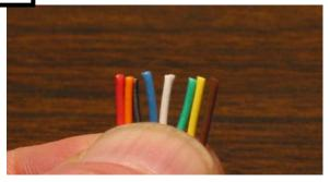
Trim the ends of the wires to make them even. This will make it easier to insert the wires into the load bar. Remove the least amount of wire necessary to even out the wires.
