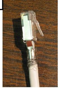
Squeeze the handles of the crimp tool together until they are fully depressed, and will open when the handle is released.
