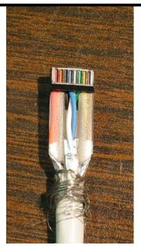
Wrap the braid over the jacket. Press the foil covered pairs fully into the slots in the channels of the plastic wire aligner. Ensure that the foil does not stick out as this makes it difficult to insert this assembly into the plug body.
