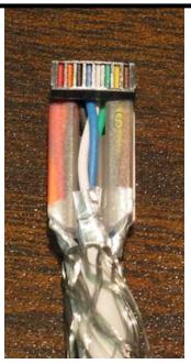
Bring the loadbar down, tight against the plastic wire aligner. Trim the wires flush to the loadbar.
