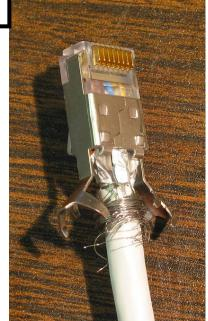
Keep the orange pair to the left and the brown to the right. Push the assembled wires, loadbar, and plastic wire aligner into the plug body subassembly. The plug latch tab should be facing away from you. Firmly push the plug until the wires come in contact with the front inside surface of the plug.
