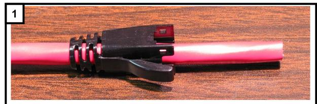
Cut cable to length. If you are using a strain relief grommet, slide it over the cable. The larger ends should be facing outward, toward the plug end of the cable.
