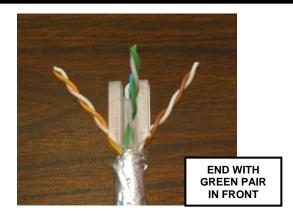
Place plastic wire aligner between the pairs. The tapered end should be toward the braid and jacket. The orange pair will go to the deep channel on the left side and the brown pair will go toward the deep channel on the right. The blue and green pairs will go to the sides that have shallow channels at the middle. On one end of the cable the blue pair will be towards you, and the green pair will be towards you on the other end.
