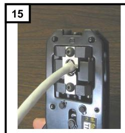
Insert the un-terminated plug into the crimp tool. Make sure that the plug is fully seated in the tool.
