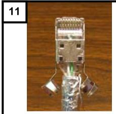
Wrap the drain wire around the foil near the wire aligner. Keep the orange pair to the left. Push the assembled wires, loadbar, and plastic wire aligner into the plug body subassembly. The plug latch tab should be facing away from you. Firmly push the plug until the wires come in contact with the front inside surface of the plug.
