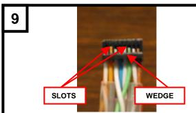
Trim the ends of the wires to make them even. This will make it easier to insert the wires into the load bar. Remove the least amount of wire necessary. Insert the ends of the wires into the wide end of the load bar, maintaining the wire color sequence. The side with the slots and the wedge shaped end should be facing towards you.
