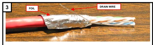
Fold the foil shield and drain wire back over the cable jacket.
