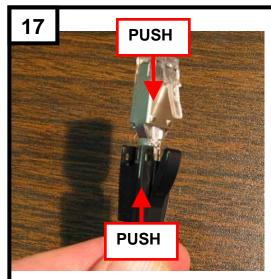
If used, align the strain relief grommet and push it over the terminated plug body. Snap it in place.
