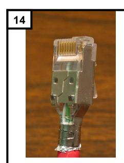
Remove the terminated plug from the crimp tool and trim off any excess foil and drain wire.
