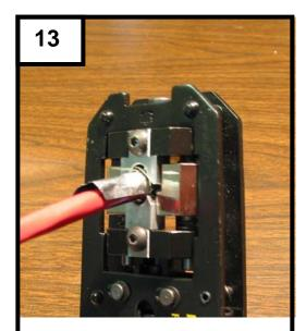
Insert the un-terminated plug into the crimp tool. Make sure that the plug is fully seated in the tool. Squeeze the handles of the crimp tool together until they are fully depressed, and will open when the handle is released.
