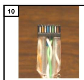
Bring the loadbar down, tight against the plastic wire aligner. Trim the wires flush to the loadbar.
