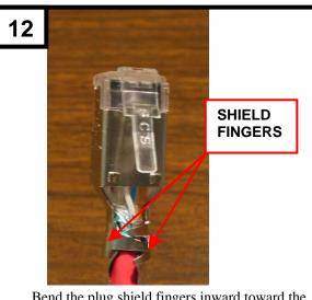
Bend the plug shield fingers inward toward the cable. Press the shield fingers as far as they will go. They should easily fit into the Shield Crimp portion of the crimping tool.
