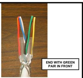
Push the wire aligner down as far as it will go and push pairs into wire aligner channels. Flatten out the wires and arrange the insulation colors so that they match the T568B color map. Keep the red on left and the brown on right. On one end of the cable the blue pair will be towards you, and the green pair will be towards you on the other end.
