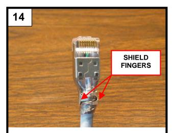
Bend the plug shield fingers inward toward the cable. Press the shield fingers as far as they will go. They should easily fit into the Shield Crimp portion of the crimping tool.
