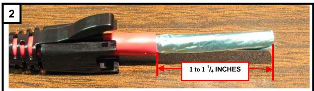
Cut and strip off 1 to  $1^{1}/_{4}$  inches of the outer jacket. Be careful not to cut or nick the drain wire and foil shield.
