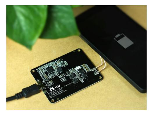
Your phone will enter the charging mode when D1 is flashing and buzzer is turned on.
