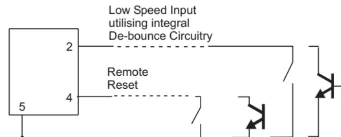
The low speed input (pin 2) should always be used for contact closure because this is the only input which contains de-bounce circuitry.
