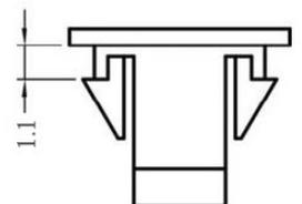
To mount  $\phi 5$  LED on board quickly.
