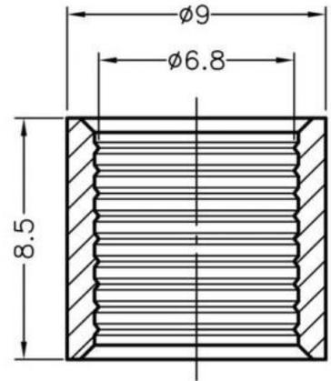
To mount  $\phi 5$  LED on board quickly. FIX-LED5-8T can be spacer or enhance and mount with FIX-LED5-8 on board.
