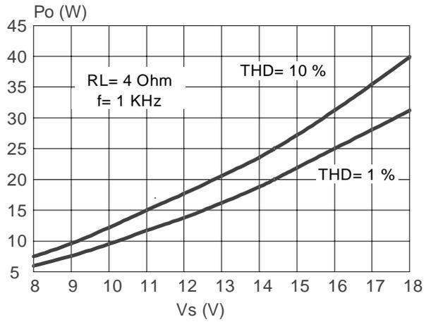
**Figure 5: Max. Output Power vs. Supply Voltage**
