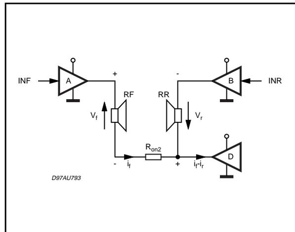
**Figure 17:** He Bridge Operation (Po < 2.5W)
