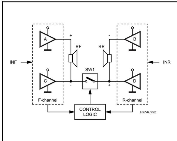
**Figure 16:** Single Ended Operation (Po < 2.5W)
