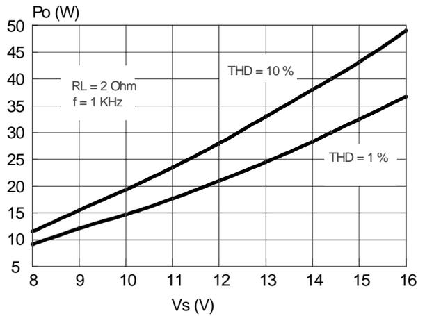
**Figure 7: Max. Output Power vs. Supply Voltage**
