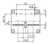
TOLERANCE; less than 10mm: ±0.3 min.10mm~ : ±0.5
