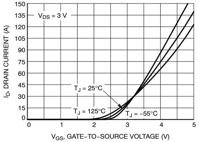
Figure 2. Transfer Characteristics
