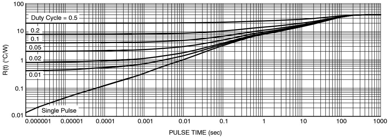
Figure 13. Thermal Characteristics
