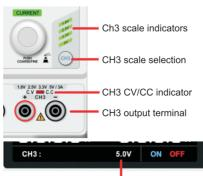
The CH3 selected voltage scale is lit on LCD
