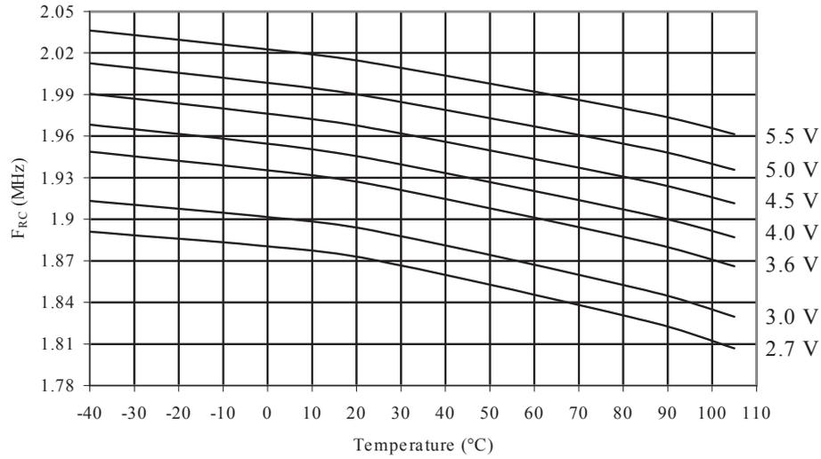
**Figure 33-44 Calibrated 2MHz RC Oscillator vs.  $V_{CC}$**
