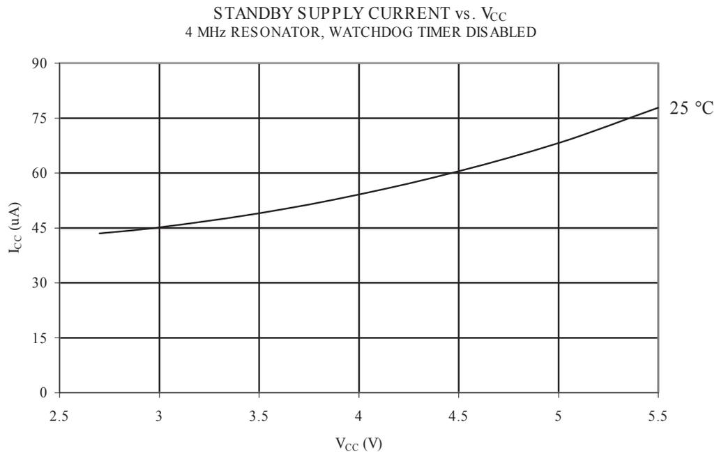
**Figure 32-21 Standby Supply Current vs.  $V_{CC}$  (4MHz Xtal, Watchdog Timer Disabled)**
