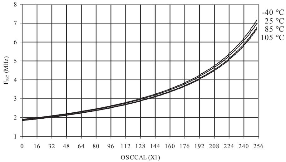
**Figure 33-43 Calibrated 2MHz RC Oscillator vs. Temperature**
