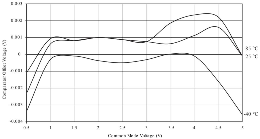
**Figure 32-49 Analog Comparator Offset Voltage vs. Common Mode Voltage ( $V_{CC} = 2.8V$ )**
