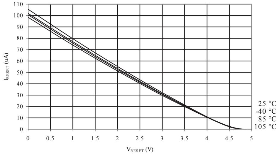
**Figure 33-17 Reset Pull-up Resistor Current vs. Reset Pin Voltage ( $V_{CC} = 2.7V$ )**
