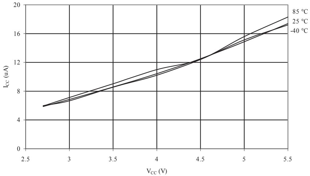
**Figure 32-68 Analog Comparator Current vs. V<sub>CC</sub>**
