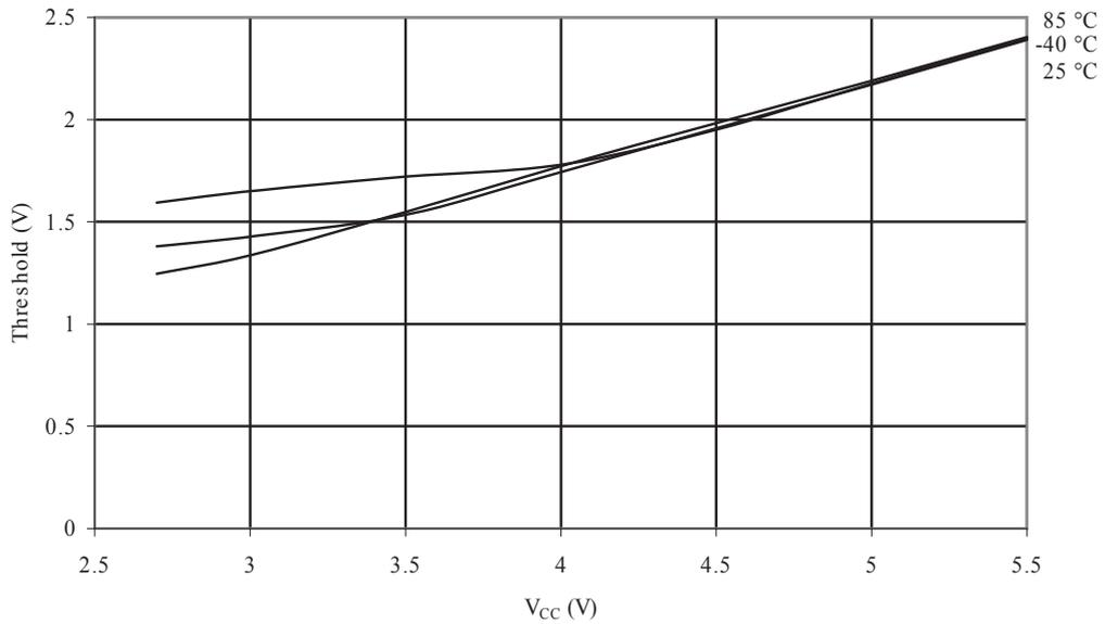
**Figure 32-43 Reset Input Threshold Voltage vs.  $V_{CC}$  ( $V_{IL}$ , Reset Pin Read as "0")**
