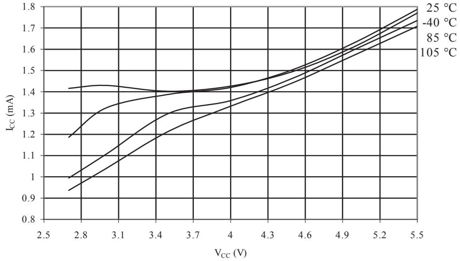
**Figure 33-5 Active Supply Current vs. V<sub>CC</sub> (32 kHz External Oscillator)**
