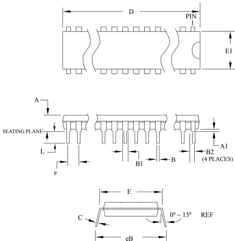
Note: 1. Dimensions D and E1 do not include mold Flash or Protrusion. Mold Flash or Protrusion shall not exceed 0.25mm (0.010").
