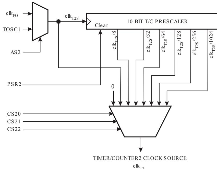
The clock source for Timer/Counter2 is named  $clk_{T2S}$ .  $clk_{T2S}$  is by default connected to the main system clock  $clk_{I/O}$ . By setting the AS2 bit in ASSR, Timer/Counter2 is asynchronously clocked from the TOSC1 pin. This enables use of Timer/Counter2 as a Real Time Counter (RTC). When AS2 is set, pins TOSC1
