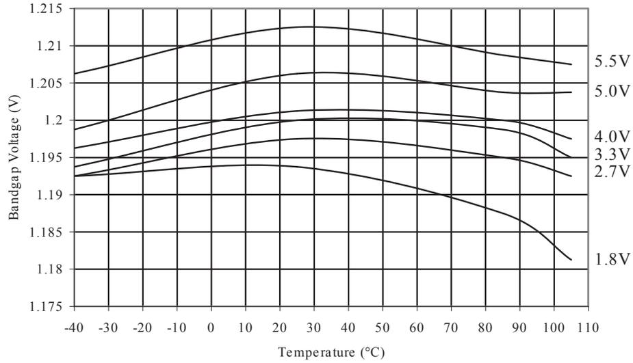
**Figure 33-34 Bandgap Voltage vs. V<sub>CC</sub>**
