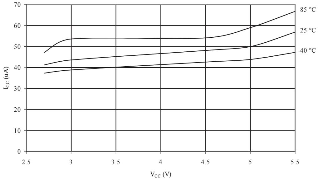
**Figure 32-69 Programming Current vs.  $V_{CC}$**
