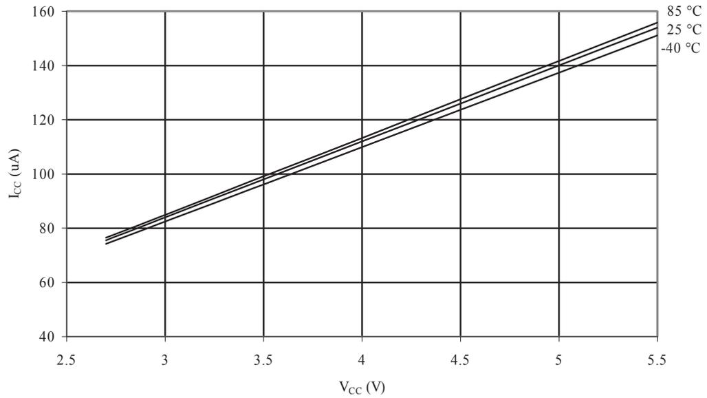
**Figure 32-66 32kHz TOSC Current vs. V<sub>CC</sub> (Watchdog Timer Disabled)**
