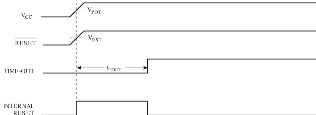
**Figure 15-3 Figure: MCU Start-up,  $\overline{\text{RESET}}$  Extended Externally**
