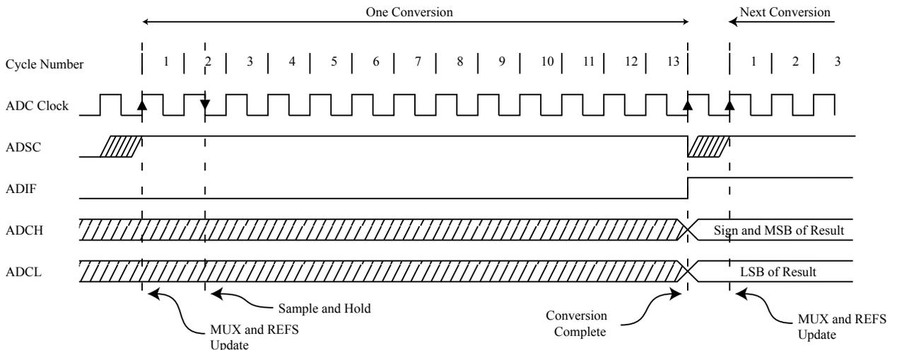
**Figure 27-5 ADC Timing Diagram, Free Running Conversion**
