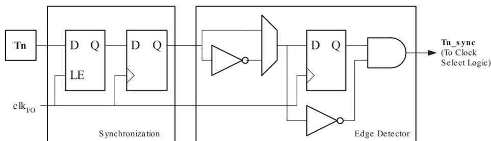
The synchronization and edge detector logic introduces a delay of 2.5 to 3.5 system clock cycles from an edge has been applied to the T1/T0 pin to the counter is updated.
