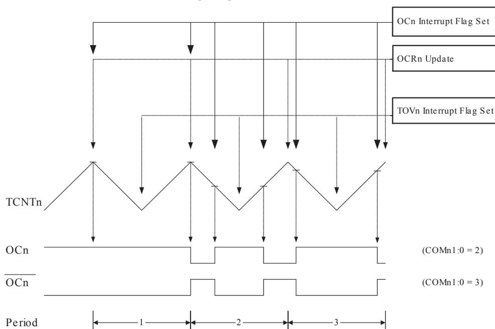
The Timer/Counter Overflow Flag (TOV2) is set each time the counter reaches BOTTOM. The Interrupt Flag can be used to generate an interrupt each time the counter reaches the BOTTOM value.
