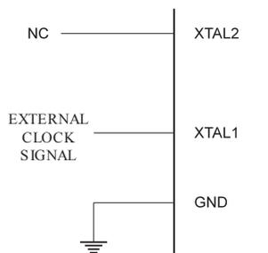
When this clock source is selected, start-up times are determined by the SUT Fuses as shown in the following table.
