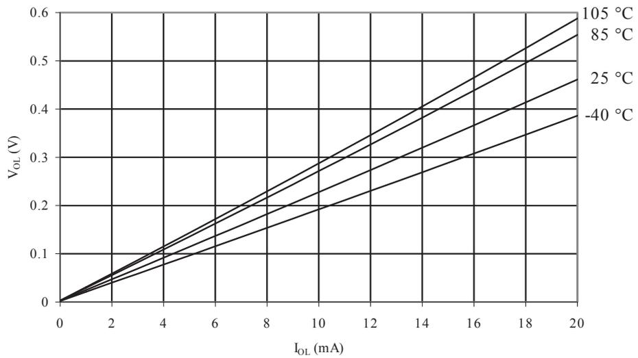
**Figure 33-21 I/O Pin Output Voltage vs. Sink Current ( $V_{CC} = 3V$ )**
