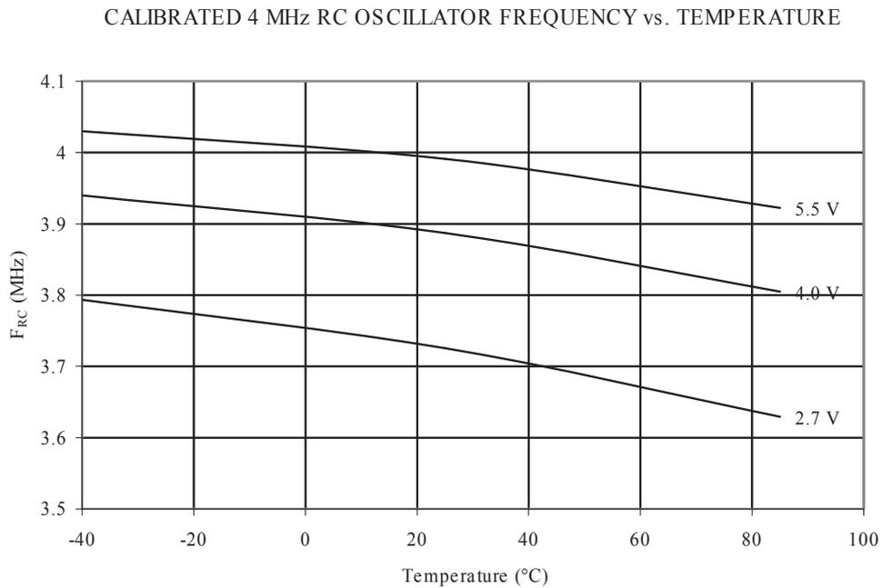
**Figure 32-55 Calibrated 4MHz RC Oscillator Frequency vs. V<sub>CC</sub>**
