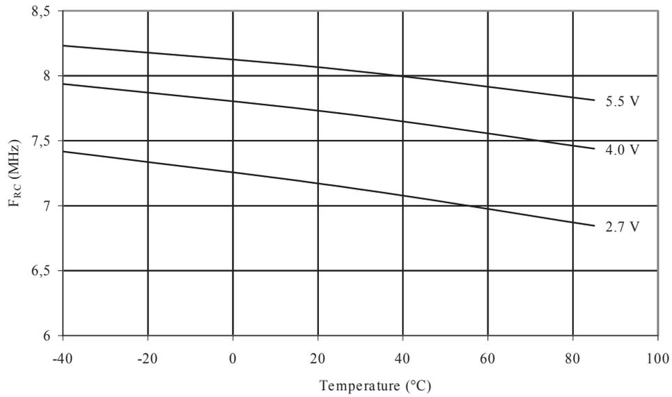
**Figure 32-52 Calibrated 8MHz RC Oscillator Frequency vs.  $V_{CC}$**
