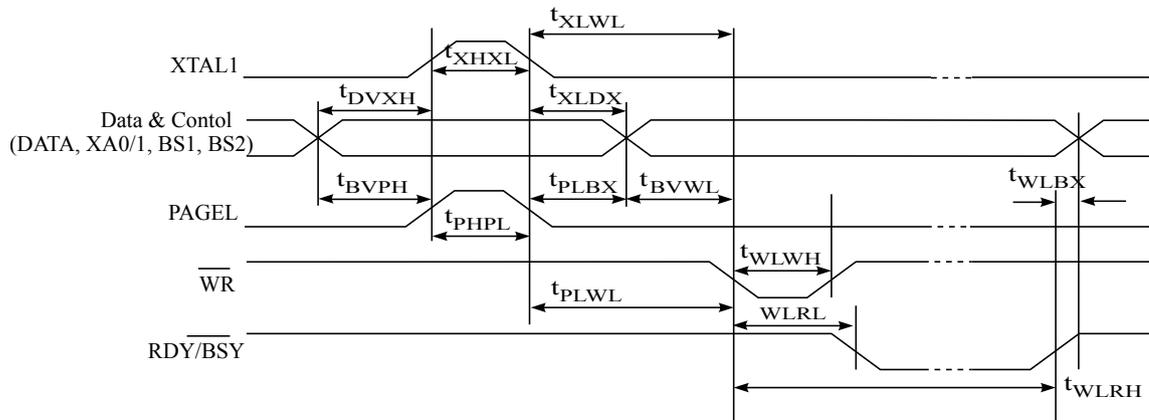
Figure 29-7 Parallel Programming Timing, Loading Sequence with Timing Requirements<sup>(1)</sup>
