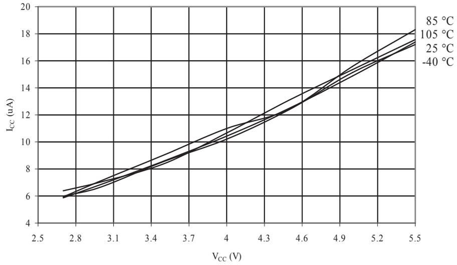
Figure 33-52 Analog Comparator Current vs.  $V_{CC}$
