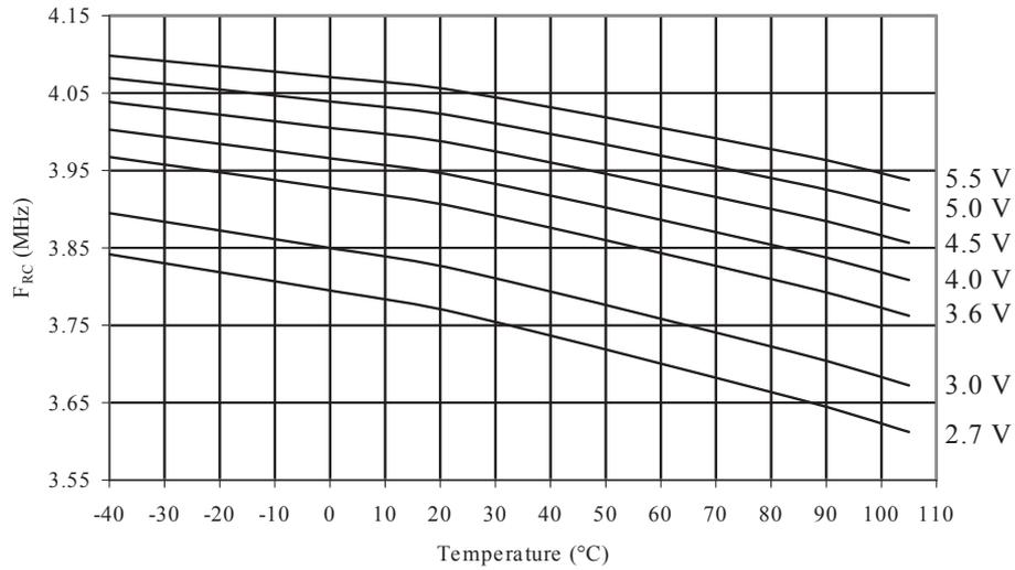
**Figure 33-41 Calibrated 4MHz RC Oscillator vs. V<sub>CC</sub>**
