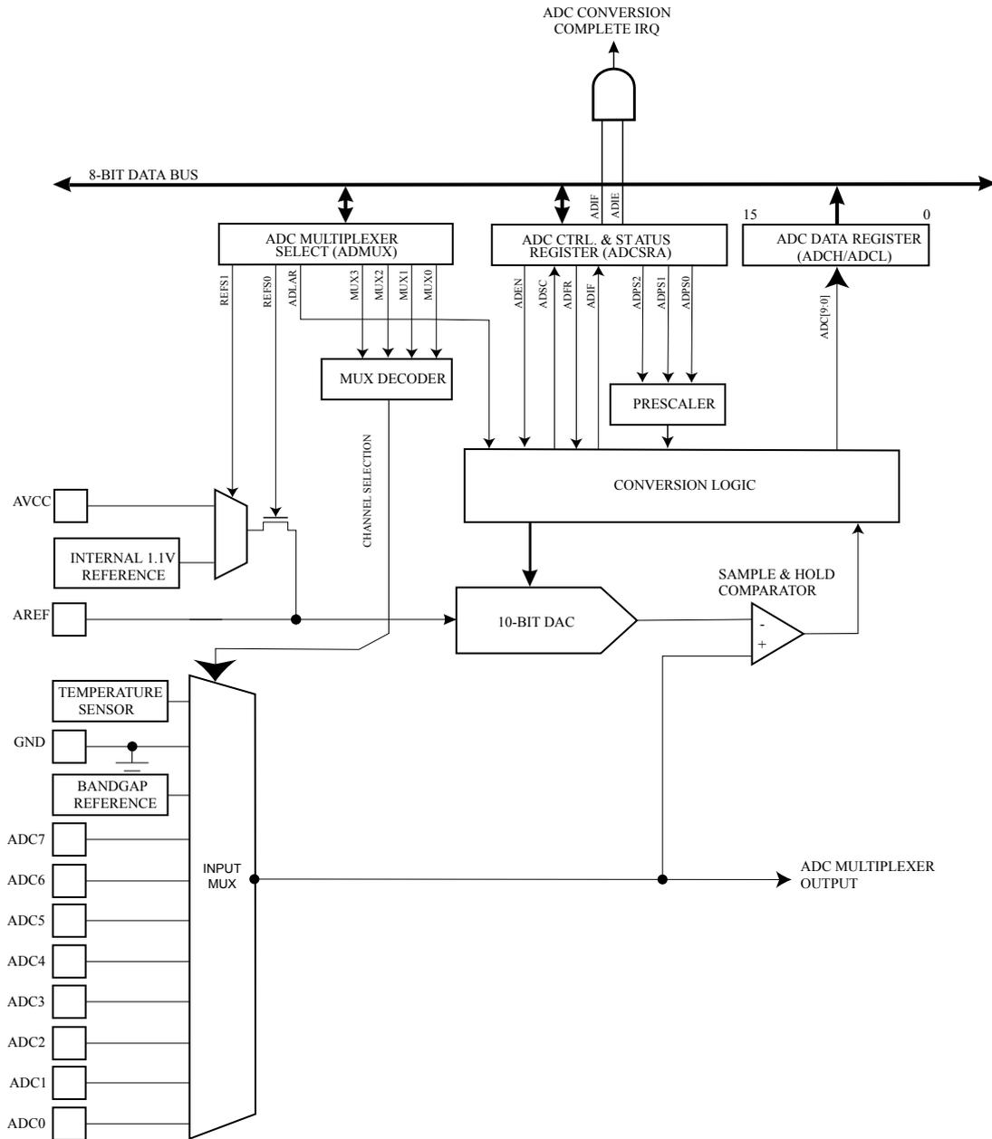
The ADC converts an analog input voltage to a 10-bit digital value through successive approximation. The minimum value represents GND and the maximum value represents the voltage on the AREF pin minus 1LSB. Optionally,  $AV_{CC}$  or an internal 2.56V reference voltage may be connected to the AREF pin by writing to the REFSn bits in the ADMUX Register. The internal voltage reference may thus be decoupled by an external capacitor at the AREF pin to improve noise immunity.
