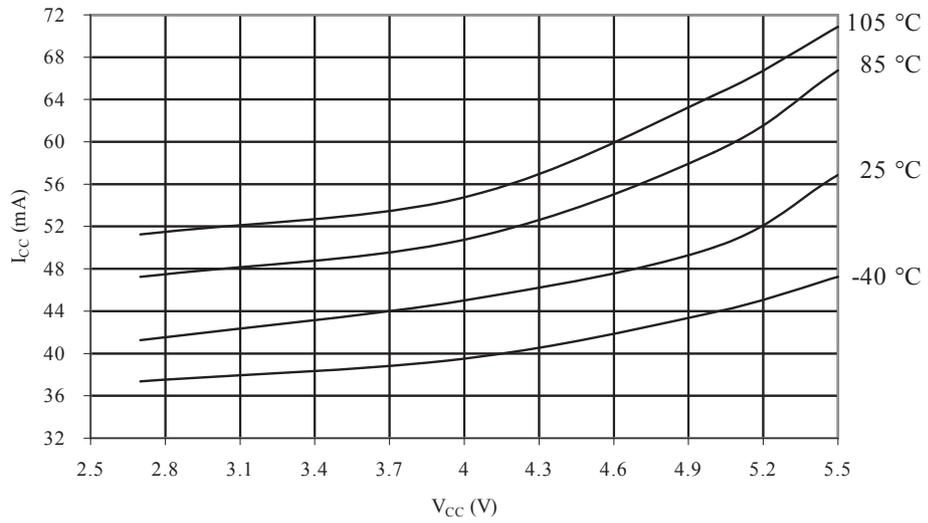
**Figure 33-53 Programming Current vs. V<sub>CC</sub>**
