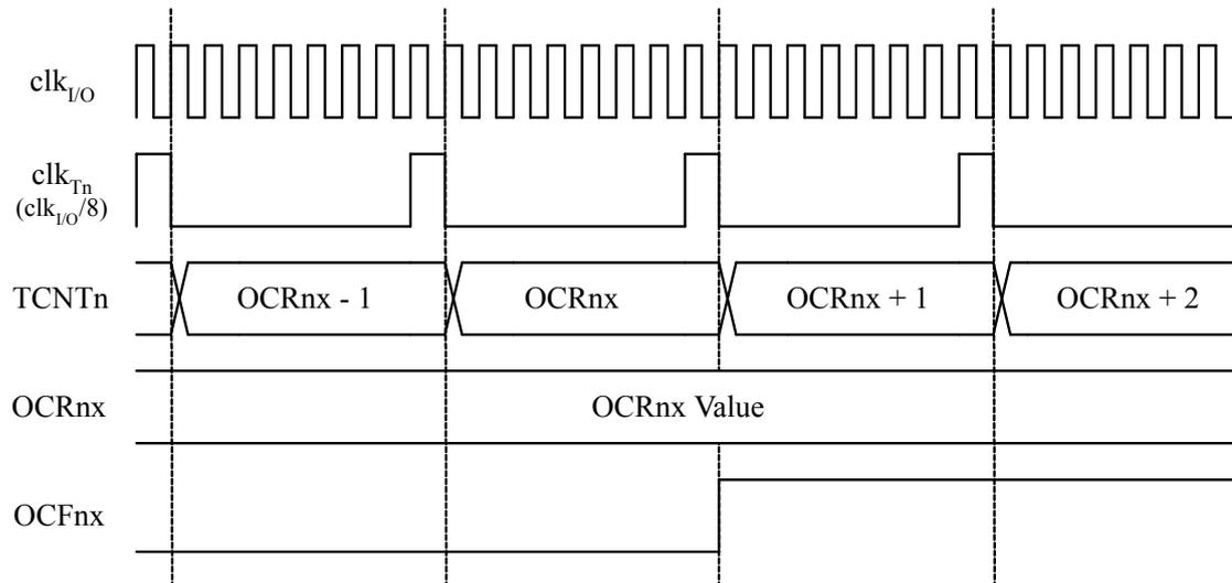
The next figure shows the count sequence close to TOP in various modes. When using phase and frequency correct PWM mode the OCR1x Register is updated at BOTTOM. The timing diagrams will be the same, but TOP should be replaced by BOTTOM, TOP-1 by BOTTOM+1 and so on. The same renaming applies for modes that set the TOV1 Flag at BOTTOM.
