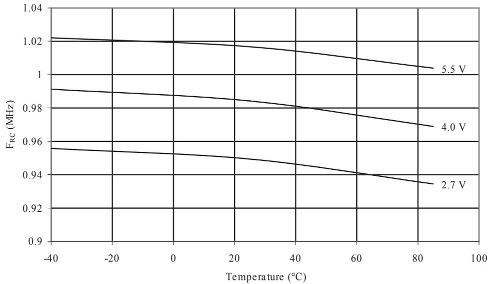
**Figure 32-61 Calibrated 1MHz RC Oscillator Frequency vs.  $V_{CC}$**
