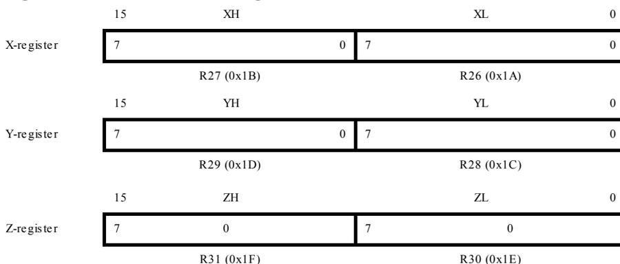
In the different addressing modes these address registers have functions as fixed displacement, automatic increment, and automatic decrement (see the Instruction Set Reference for details).
