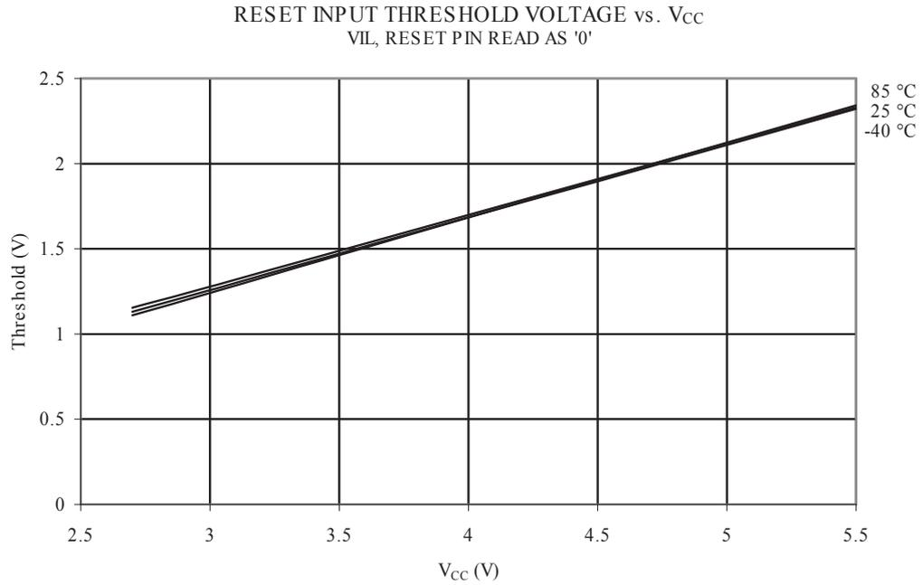
**Figure 32-44 Reset Input Pin Hysteresis vs.  $V_{CC}$**
