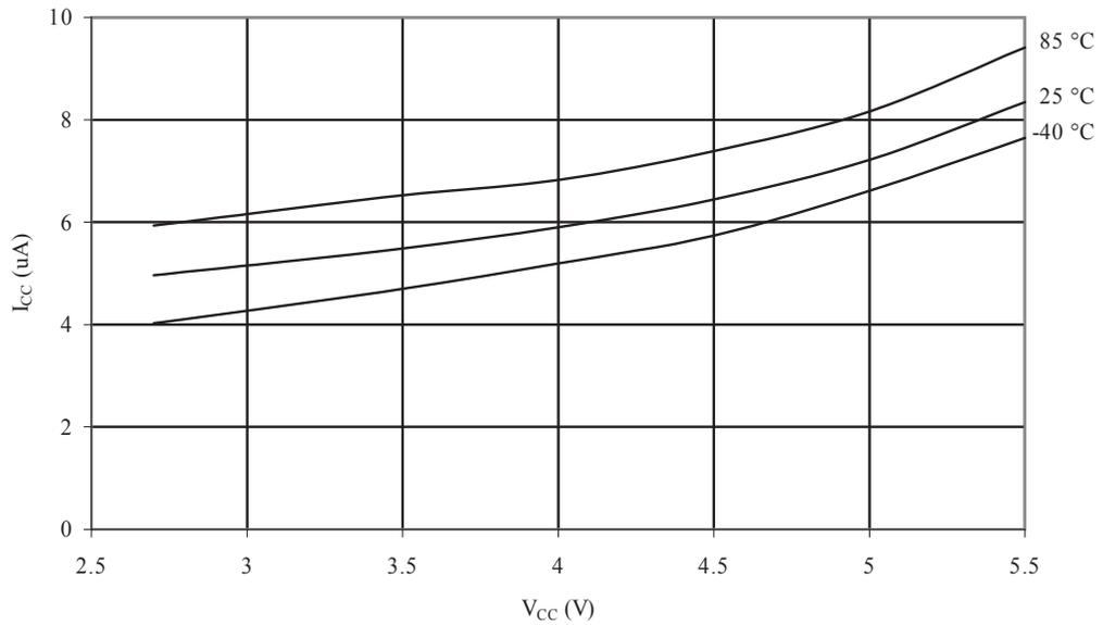
**Figure 32-67 Watchdog Timer Current vs. V<sub>CC</sub>**
