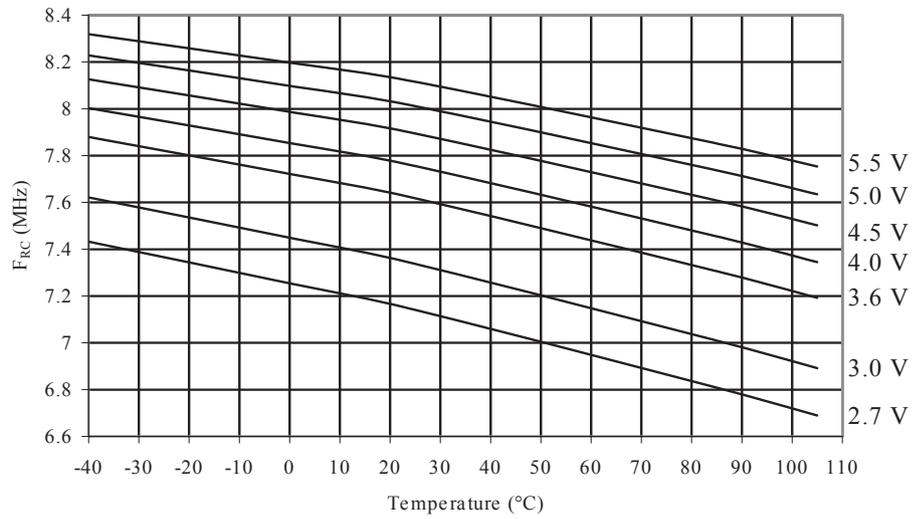
**Figure 33-38 Calibrated 8MHz RC Oscillator vs.  $V_{CC}$**
