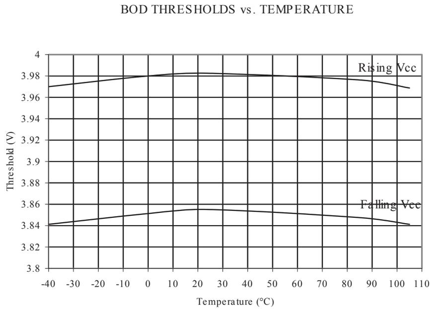
Figure 33-32 BOD Threshold vs. Temperature ( $V_{CC} = 2.7V$ )
