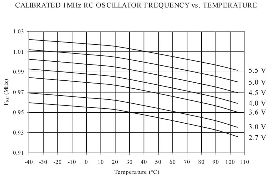
**Figure 33-47 Calibrated 1MHz RC Oscillator vs. V<sub>CC</sub>**
