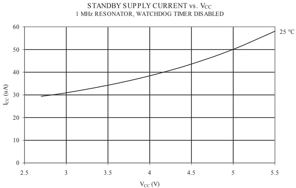
**Figure 32-19 Standby Supply Current vs.  $V_{CC}$  (1MHz Xtal, Watchdog Timer Disabled)**
