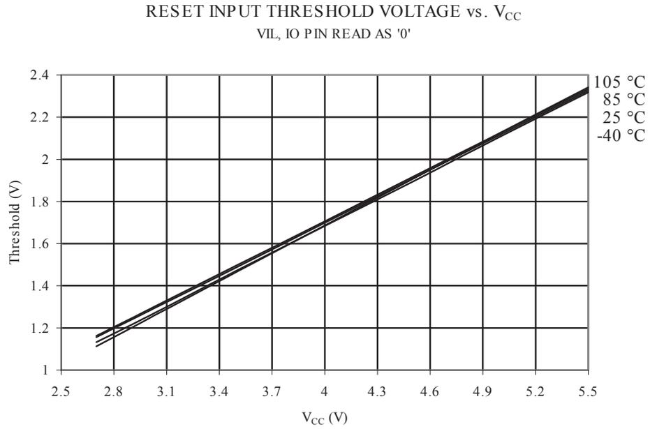
**Figure 33-30 Reset Pin Input Hysteresis vs.  $V_{CC}$**
