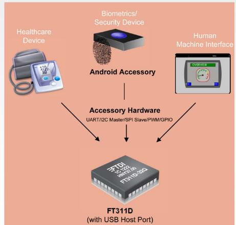
**USB Connection providing data connectivity**
