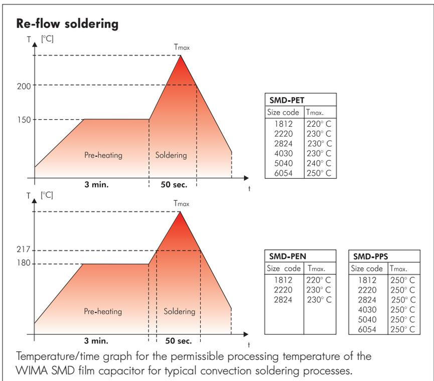
Due to versatile procedures exact processing parameters for re-flow soldering processes cannot be specified. The graph depicted is to be understood as a recommendation to help establishing a suitable soldering profile fulfilling the requirements
