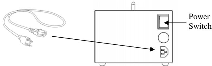
2. Switch on the main power switch to turn unit ON.
