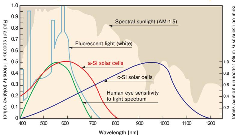
Light wavelength differs depending on the light sources to which they are exposed. Spectral sensitivity of solar cells also differs depending on the category. Amorphous silicon solar cells provide light-sensing capability similar to the human eye.
