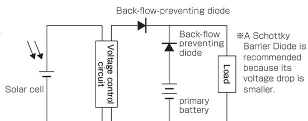
※A Schottky Barrier Diode is recommended because its voltage drop is smaller.
