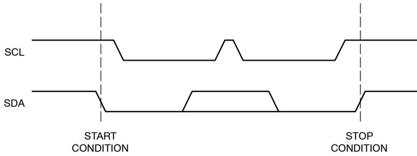
**Figure 2. Start/Stop Timing**
