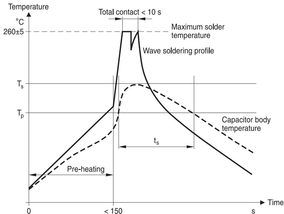
$T_s$ : Capacitor body maximum temperature at wave soldering
