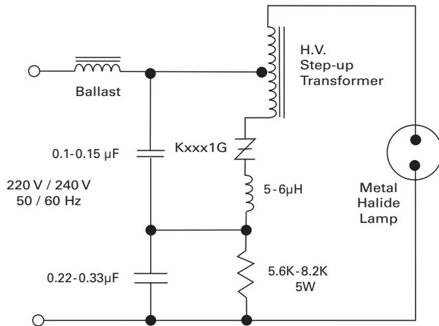
Note: With proper component selection, this circuit will produce three pulses for ignition of metal halide lamp that requires a minimum of three pulses at 4kV magnitude and >1uSec duration each at a minimum repetition rate of 3.3kHz.
