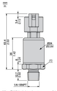
(1) SW24, tightening torque  $\leqslant$  24 N-m / 212 lb-in
