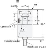
Robot cable of 2.8 dia., 4 cores, (0.15 mm² with 0.8 mm dia. insulator); Standard length: 1 m
