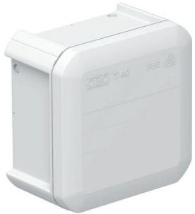
All the T series junction boxes are UV-resistant. They are made from polypropylene (a thermoplastic material) and have closed side walls. This means that the required openings can be made wherever they are required. EDK plug-in seals or cable glands with locknuts can be  $\,$ inserted in these openings, to allow cable insertion.
