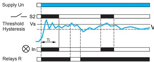
On energization, in order to allow the process being monitored to reach its nominal operating speed, relay RM35S is inhibited for a time delay adjustable from 0.6...60 s. This time delay can be modified (shortened or lengthened) during inhibition.
