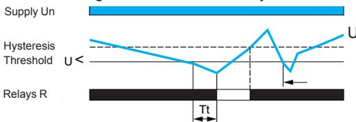
If the controlled voltage falls below the threshold setting for a time greater than that set on the front panel (0.1...10 s), the output relay opens and the R LED goes off. As soon as the voltage returns to a value above (or below) the threshold setting minus (or respectively plus) the hysteresis, the relay instantly closes.
