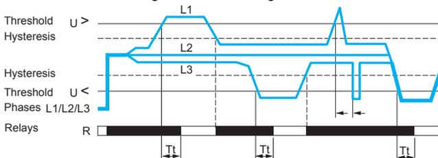
Tt: time delay after crossing of the threshold (adjustable on front panel)
