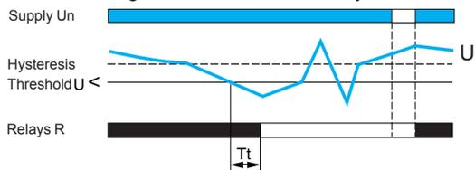
**Note:**  $T_t$ : time delay after crossing of the threshold (adjustable on front panel)
