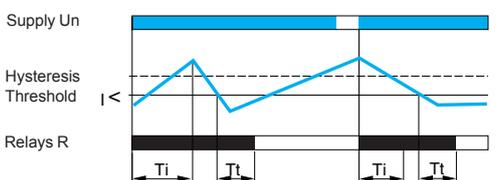
**Note:**  $T_i$ : starting inhibition time (adjustable on front panel)
