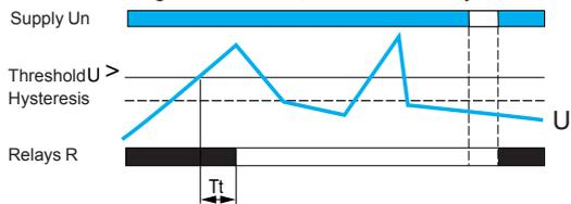
If "Memory" mode is selected, the relay opens when crossing of the threshold is detected and then stays in that position. The power needs to be switched off to reset the product.
