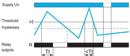
If the controlled current exceeds the threshold setting for a time greater than that set on the front panel (0.1...30 s), the output relay opens and the R LED goes off. During the time delay, this LED flashes.
