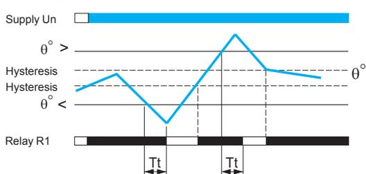
After a delay on pick-up after energization, and for as long as the temperature monitored by the PT100 probe remains between the two threshold settings on the front panel, the temperature relay R1 is closed.
