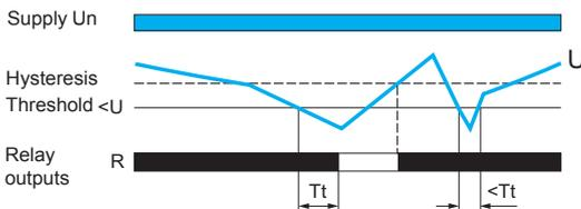
If the controlled voltage falls below the threshold setting for a time greater than that set on the front panel (0.1...30 s), the output relay opens and the R LED goes off. During the time delay, this LED flashes.
