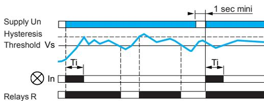
At the end of the starting inhibition time delay “Ti”, as soon as the speed measured drops below the threshold setting, the output relay changes state from “closed” to “open”.
