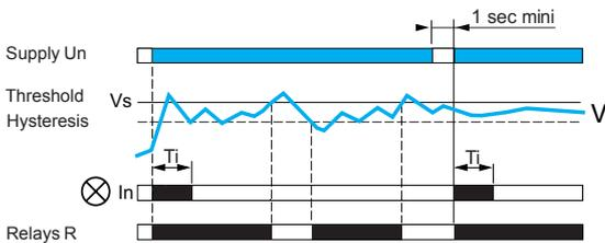
At the end of the starting inhibition time delay, “Ti”, as soon as the speed measured is higher than the threshold setting, the output relay changes state from “closed” to “open”.
