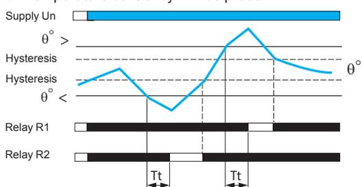
After a delay on pick-up after energization, and for as long as the temperature monitored by the PT100 probe remains between the two threshold settings on the front panel, the output relays are closed and their yellow LEDs are on.
