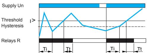
If "Memory" mode is selected, the relay opens when crossing of the threshold is detected and then stays in that position. The power needs to be switched off to reset the product.
