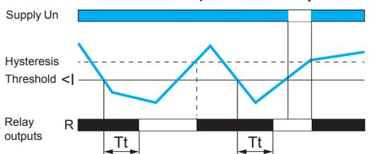
If the controlled current falls below the threshold setting for a time greater than that set on the front panel (0.1...30 s), the output relay opens and the R LED goes off. During the time delay, this LED flashes.
