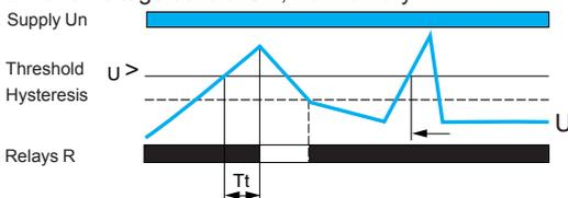
If the controlled voltage exceeds the threshold setting for a time greater than that set on the front panel (0.1...10 s), the output relay opens and the R LED goes off. As soon as the voltage returns to a value below the threshold setting plus the hysteresis, the relay instantly closes.
