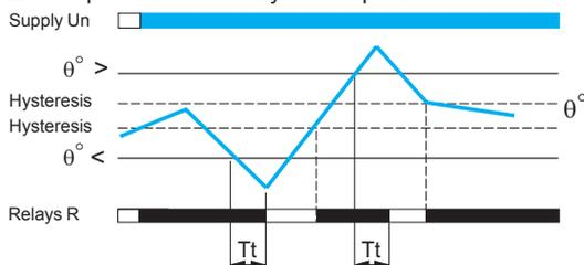
After a delay on pick-up after energization, and for as long as the temperature monitored by the PT100 probe remains between the two thresholds set on the front panel, the output relay is closed and the yellow LEDs are on.
