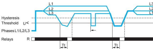
Tt: time delay after crossing of the threshold (adjustable on front panel)
