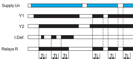
This mode is designed to control a pump via two external control signals (Y1 and Y2). The output relay closes when both input signals are present (Y1 and Y2 closed). It will open as soon as one of these signals disappears.
