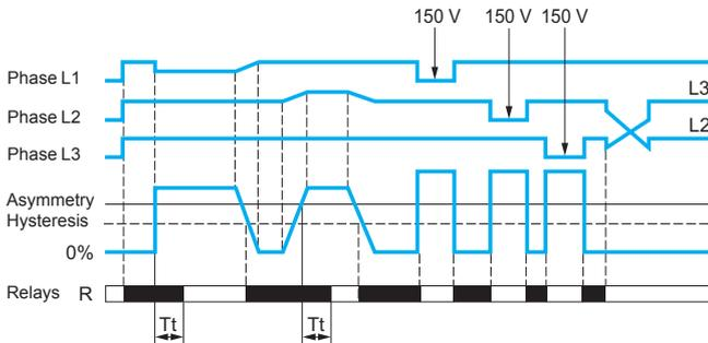
Tt: time delay after crossing of the threshold (adjustable on front panel)
