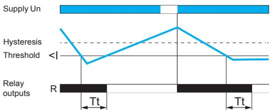
**Note:**  $T_t$ : time delay after crossing of the threshold
