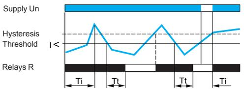
If the current controlled falls below the threshold setting for a time greater than that set on the front panel (0.3...30 s), the output relay opens and the LED goes off. As soon as the current rises above the value of the threshold setting plus the hysteresis, the relay instantly closes.
