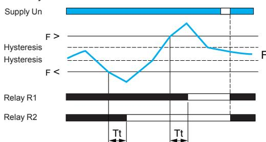
If "Memory" mode is selected, the relay opens after the time delay and stays in that position when crossing of the threshold is detected. The power needs to be switched off to reset the product.
