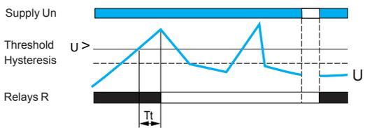
**Note:**  $T_t$ : time delay after crossing of the threshold
