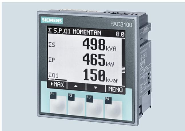
The 7KM PAC measuring devices are used to measure and display all relevant system parameters in low-voltage power distribution. They can be used for both single-phase and multi-phase measurements in 3 and 4-conductor power supply systems (TN, TT, IT).
