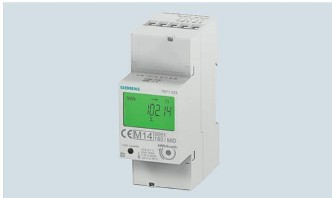
The 7KT PAC1500 single-phase measuring devices (power meters) are used to record the amount of electrical energy and power exported and imported. They comply with the metering equipment standard EN 50470 (Part 1 and 3) and come with an LCD display.
