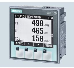
The 7KM PAC measuring devices are used to measure and display all relevant system parameters in low-voltage power distribution. They can be used for both single-phase and multiphase measurements in 3 and 4-conductor power supply systems (TN, TT, IT).
