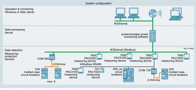
Typical topology of a power monitoring system
