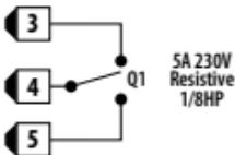
Capacity 5 A / 250 VAC for resistive loads.
