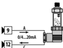
For signals 0/4..20mA with **two-wire sensor**
