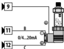
For signals 0/4..20mA with **three-wire sensor**
