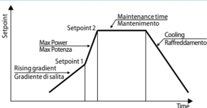
Cycle starts at each activation of the controller, or via digital input if it is enabled for this type of functioning (parameters 94 d.1.F, or 101 d.1.F set as St./St. or Rul).
