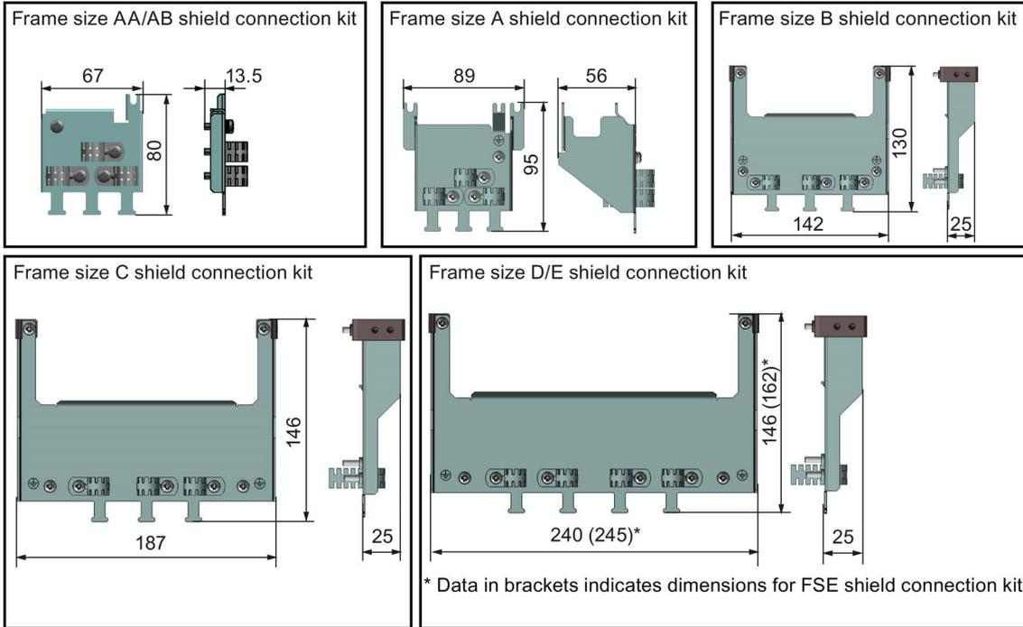
Fixing the shield connection kit to the inverter
