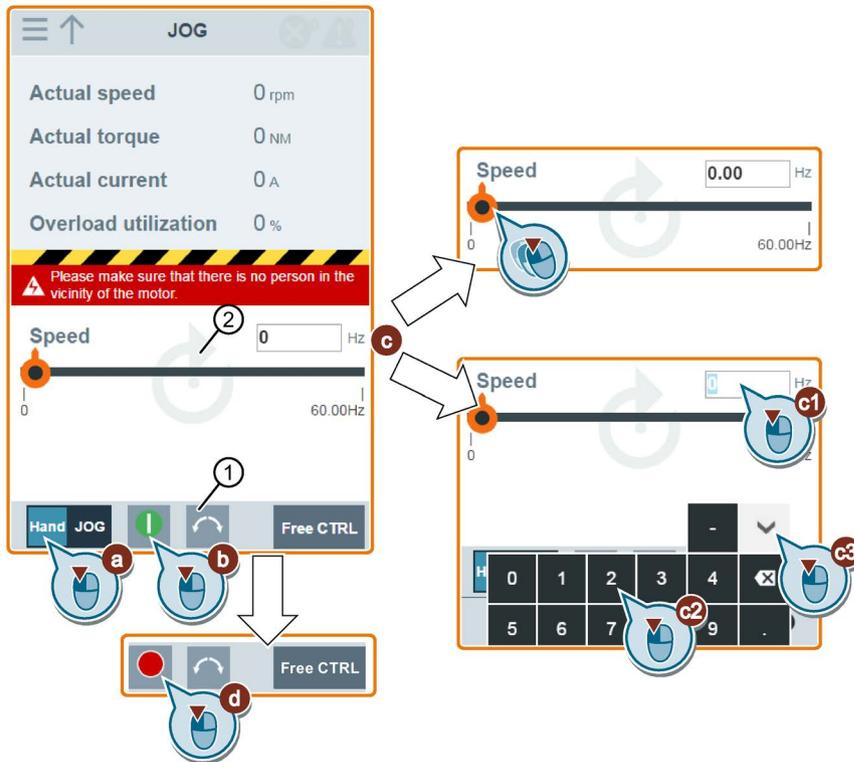
4. After you finish the motor test run, proceed as follows to return the control of the motor:
