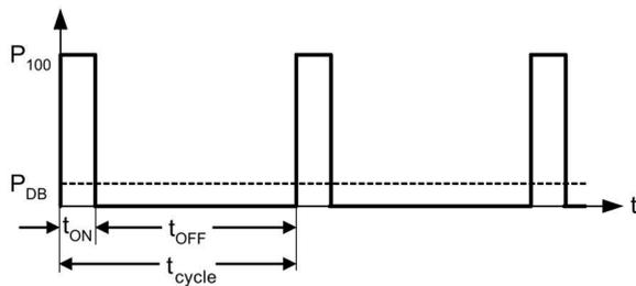
Dynamic braking switch-on level:
