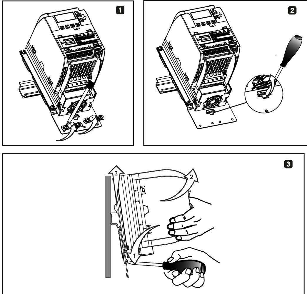
Installing FSB to the DIN rail
