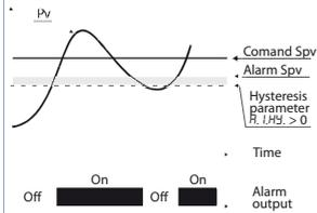
Upper deviation alarm value of alarm setpoint less than "0" and hysteresis value greater than "0" (Par.128  $R.I.H.Y. > 0$ ).
