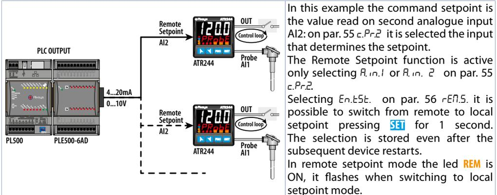
The decimal point setting parameter for the image input (or remote setpoint) is locked and modifies automatically when the command input decimal point is changed.
