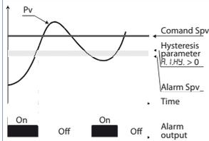
Lower deviation alarm value of alarm setpoint greater than "0" and hysteresis value greater than "0" (Par.128  $R.I.H.Y. > 0$ ).
