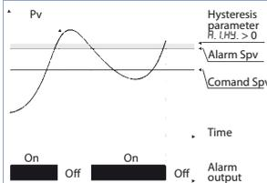
Lower deviation alarm value of alarm setpoint less than "0" and hysteresis value greater than "0" (Par.128  $R.I.H.Y. > 0$ ).
